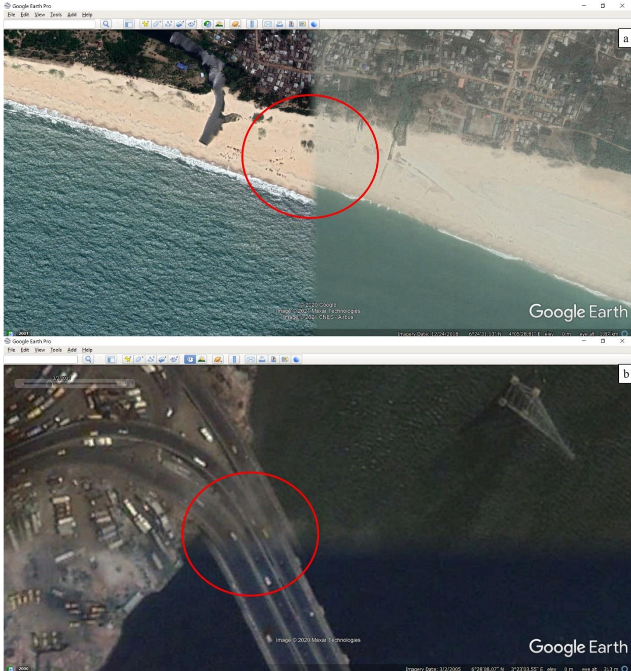
Figure 2: Region of image misalignment (within the red circles) on Google Earth imagery in Lagos, Nigeria - (a) disjoint shoreline, imagery date - December 2018 (b) disjoint roads along Carter Bridge, imagery date – March 2005
