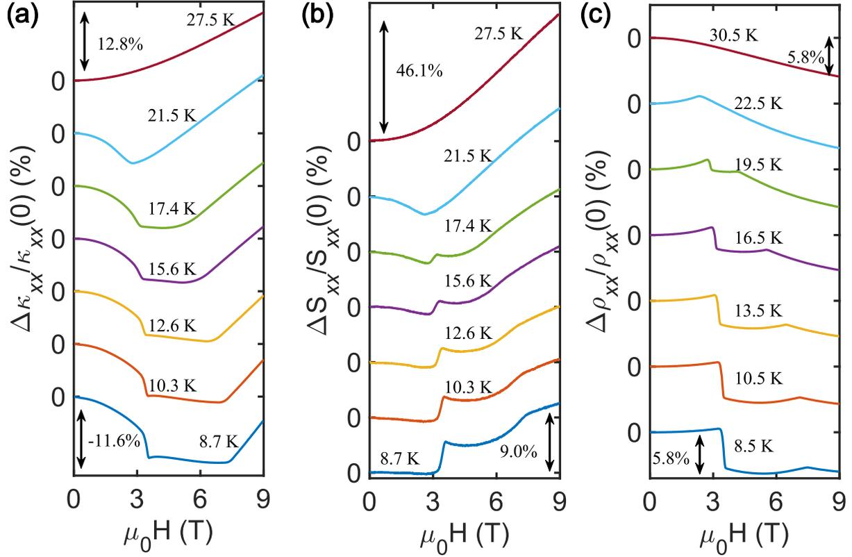
**Figure 3.** The magnetic field dependence of relative change in longitudinal (a) thermal conductivity  $\kappa_{xx}$ , (b) Seebeck coefficients  $S_{xx}$ , and (c) resistivity  $\rho_{xx}$  measured at various temperatures.
