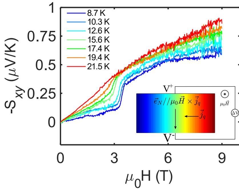
**Figure 4.** Magnetic field dependence of Nernst coefficients of  $\text{MnBi}_2\text{Te}_4$  measured at various temperatures. The inset shows a schematic of the experimental set-up.
