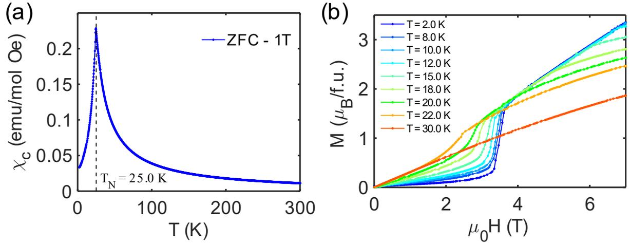
**Figure 1.** (a) Temperature dependence of magnetic susceptibility of  $\text{MnBi}_2\text{Te}_4$  measured with a 1T magnetic field applied along the crystalline  $c$ -axis. The sample is cooled under zero-field conditions. (b) Isothermal magnetization measurement of  $\text{MnBi}_2\text{Te}_4$  at various temperatures from 2 K to 30 K.
