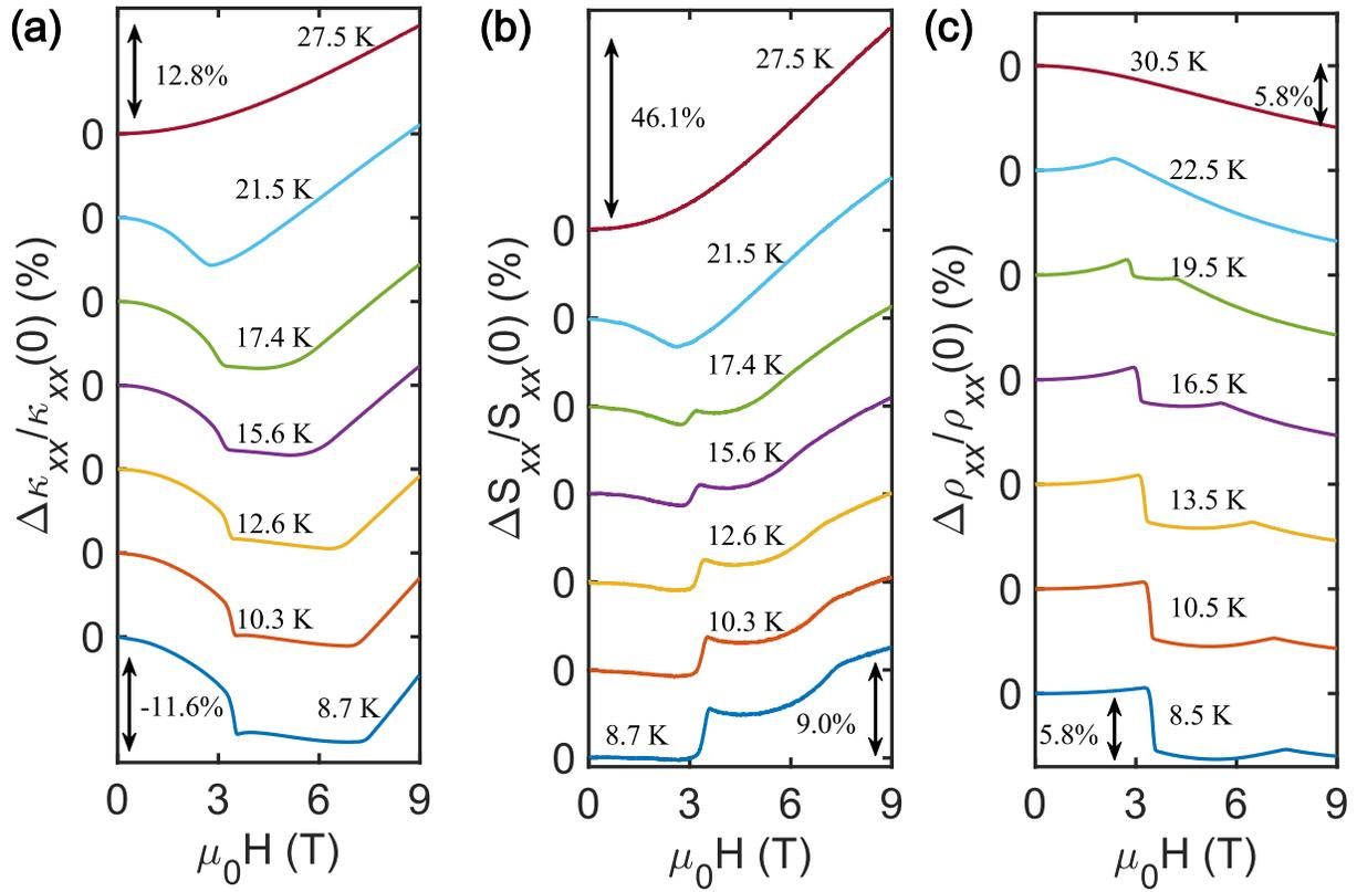
**Figure 3.** The magnetic field dependence of relative change in longitudinal (a) thermal conductivity  $\kappa_{xx}$ , (b) Seebeck coefficients  $S_{xx}$ , and (c) resistivity  $\rho_{xx}$  measured at various temperatures.
