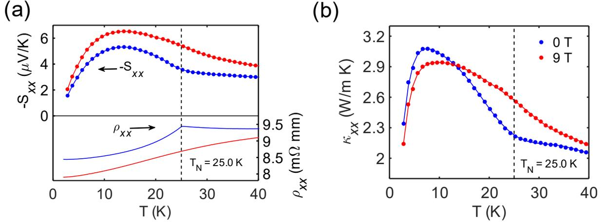
**Figure 2.** (a) Temperature dependence of longitudinal Seebeck coefficient  $S_{xx}$  (upper panel) and resistivity  $\rho_{xx}$  (lower panel) of MnBi<sub>2</sub>Te<sub>4</sub> measured under an applied field of 0 T (in blue) and 9 T (in red,  $H//c$ ). (b) Temperature dependence of longitudinal thermal conductivity  $\kappa_{xx}$  measured under an applied field of 0 T (in blue) and 9 T (in red,  $H//c$ ).
