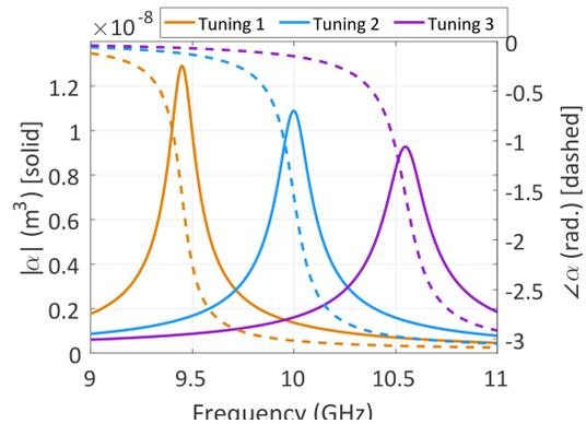
FIG. 2. Lorentzian polarizability for the idealized metamaterial element used to model a sample metasurface antenna. The three colors correspond to three different tuning states. The solid lines plot  $|\alpha|$ , while the dashed lines plot  $\angle\alpha$
