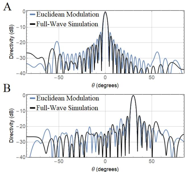
FIG. 12. Analytical (Euclidean modulation) and simulated directivity patterns (a) broadside radiation (b) steered to 30 degrees.
