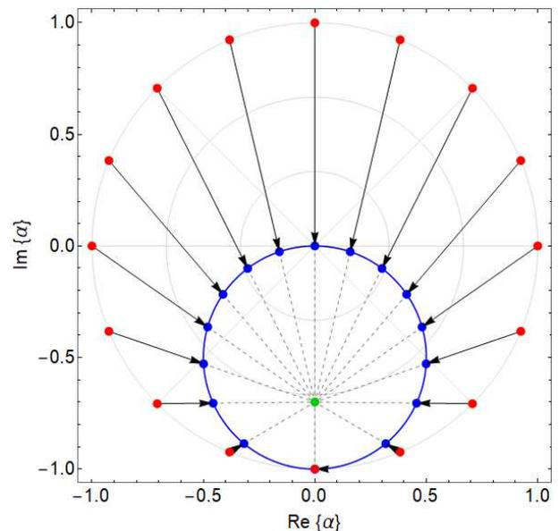
FIG. 4. Mapping between ideal polarizabilities (shown as red dots) required to achieve a directive beam and the available Lorentzian-constrained values (blue circle) for  $y_0 = -0.7$ .
