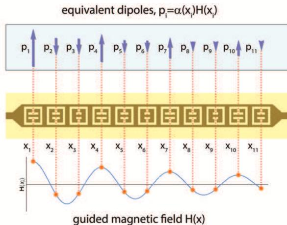
FIG. 1. Illustration of the waveguide-fed metasurface antenna. A guided wave feeds the metamaterial elements patterned in the upper conductor. Each metamaterial element scatters to good approximation as a polarizable dipole, such that the radiation can be modeled as the sum from a discrete set of dipoles.
