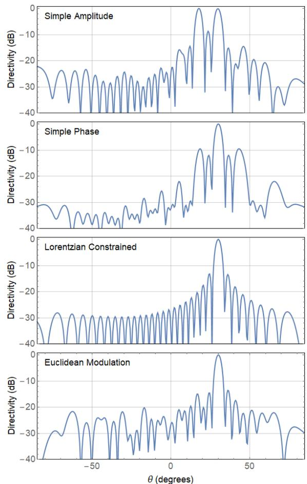
FIG. 10. Far-field radiation patterns for a beam steered to 30 degrees, optimized using the Lorentzian-constrained amplitude hologram, the Lorentzian-constrained phase hologram ( $y_0 = 0$ ), the  $y_0 = -1$  mapping, and the  $y_0 = -0.5$  mapping (Euclidean modulation).
