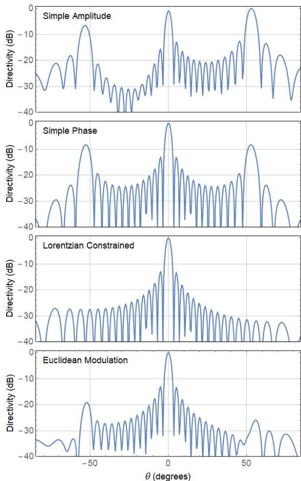
FIG. 9. Far-field radiation patterns for broadside beams optimized using the Lorentzian-constrained amplitude hologram, the Lorentzian-constrained phase hologram ( $y_0 = 0$ ), the  $y_0 = -1$  mapping, and the  $y_0 = -0.5$  mapping (Euclidean modulation).
