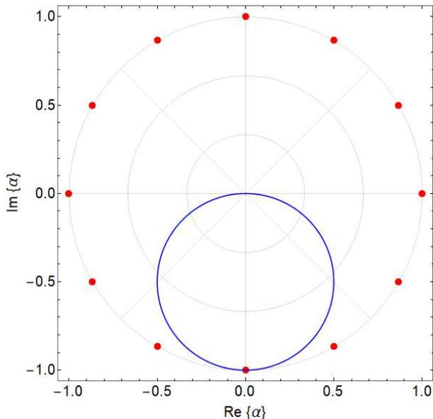
FIG. 3. Desired polarizabilities (shown as red dots) required to achieve a directive beam and the Lorentzian constrained region (blue circle) achievable by tuning metasurface elements. The axes are scaled in units of  $FQ$ .
