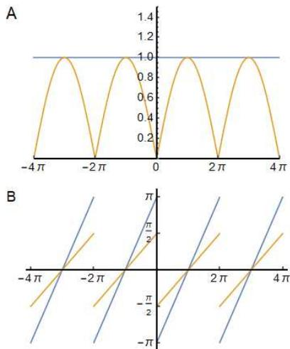
FIG. 7. (A) Amplitude and (B) phase of the Lorentzian-constrained polarizability (orange). The ideal amplitude and phase are shown for comparison as the blue curves. Note that the ideal phase has been shifted by  $\pi$  to facilitate a direct comparison.
