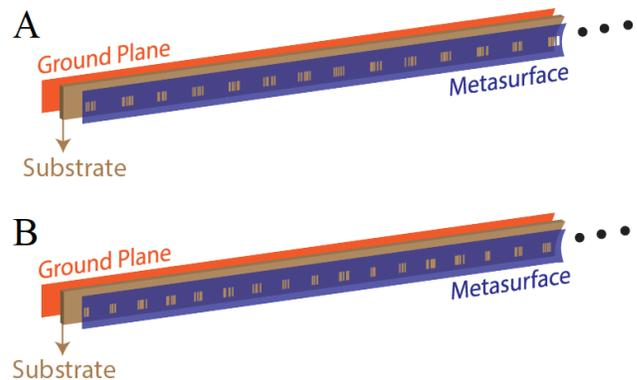
FIG. 11. Simulated metasurface antenna (a) broadside radiation (b) steered to 30 degrees. Only a portion of the metasurface antenna is shown to improve figure clarity.
