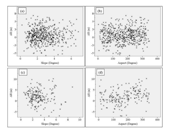
Figure 8: Variability of slope and aspect with height differences, (a) Lagos - slope (b) Lagos - aspect (c) FCT - slope (d) FCT - aspect
