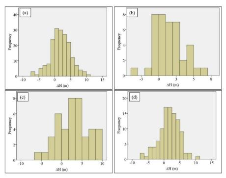
Figure 5: Histogram of height differences at FCT (a) All points (b) Bare land (c) Built-up area (d) Vegetation
