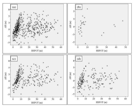
Figure 6: Plots of height differences ( $\Delta H$ ) against heights from SPOT DEM (H<sub>SPOT</sub>) at Lagos (a) All points (b) Bare land (c) Built-up area (d) Vegetation
