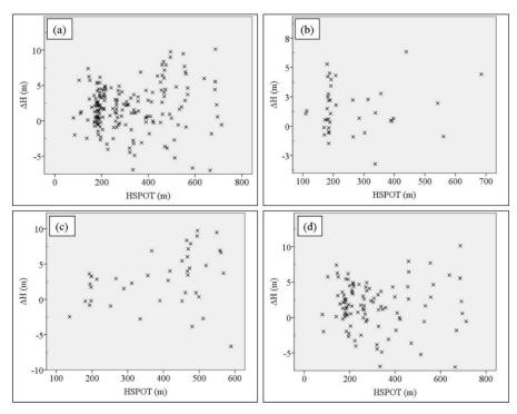
Figure 7: Plots of height differences ( $\Delta H$ ) against heights from SPOT DEM (H<sub>SPOT</sub>) at FCT (a) All points (b) Bare land (c) Built-up area (d) Vegetation
