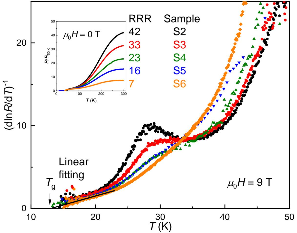
Figure 2. The temperature dependent  $(d \ln R / d T)^{-1}$  curves for a series of high- $T_c$  (43.2 – 42.1 K) (Li,Fe)OHFeSe films (S2 – S6) with different individual  $RRR = R_{300 \text{ K}} / R_{50 \text{ K}}$  values (42 – 7). The data are measured under a fixed field of 9 T. The inset shows the zero-field  $R(T) / R_{50 \text{ K}}$  curves up to  $T = 300 \text{ K}$  for the samples.
