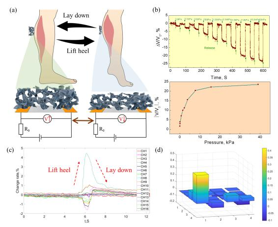
**Fig. 2. Response of the sensor array to pressures.** (a) Mechanism of sponge-based sensor detecting muscle deformation. (b) Response of individual sensory element to different applied pressure. (c) Response of all sixteen channels to the motions of lift hell and lay down with time. (d) Distribution of the mean value of rate of signal output change of the sensor array.
