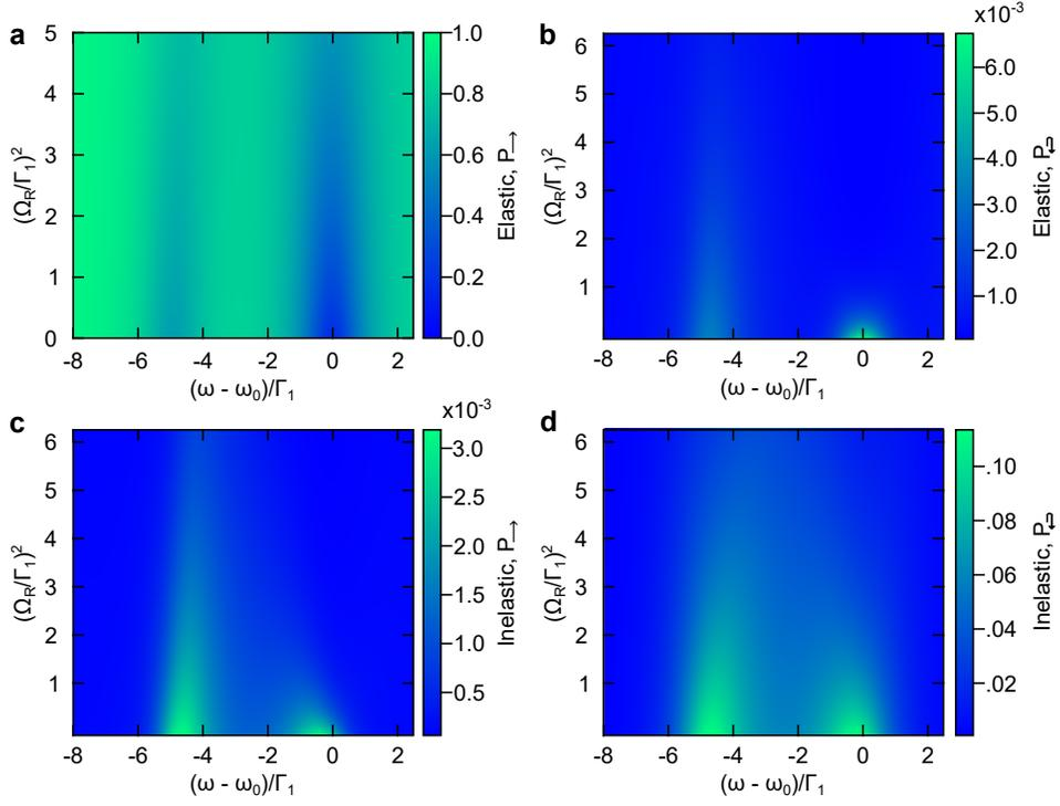
FIG. 6. **Dynamic range of directional scattering.** Calculated coherent elastic (a, b) and inelastic (c, d) scattering spectra as a function of normalized drive frequency  $(\omega - \omega_0)/\Gamma_1$  and drive power  $(\Omega_R/\Gamma_1)^2$  theoretically predicted for reflection (a, c) and transmission (b, d). The calculation has been performed for the modulation phase difference  $\alpha_2 - \alpha_1 = \pi$  and  $\Omega = A_m = 5\Gamma_1$ .
