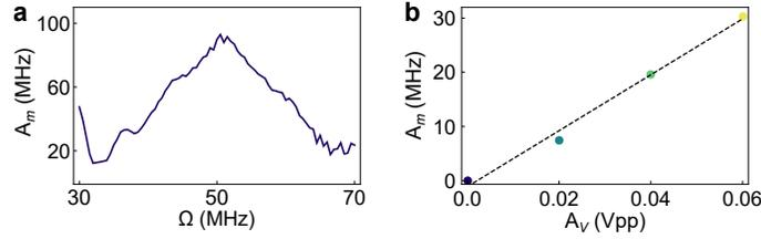
FIG. 7. **Modulation amplitude calibration.** a, Measured dependence of the modulation amplitude  $A_m$  on the modulation frequency  $\Omega$  at the fixed AWG amplitude  $A_V = 0.2 V_{pp}$ . b, Measured dependence of the modulation amplitude  $A_m$  on the applied AWG amplitude  $A_V$  at the modulation frequency  $\Omega = 20$  MHz.
