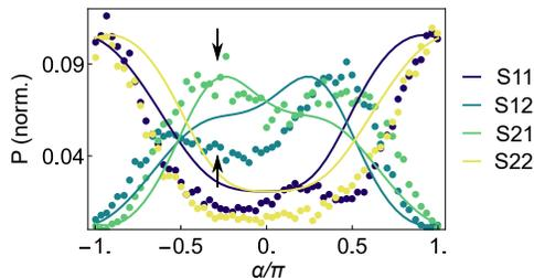
FIG. 5. **Isolator scattering matrix.** Measured coherent inelastic scattering power of the Stokes component is normalized to theory and shown as a function of the relative phase between modulation tones  $\alpha$  at  $(\omega - \omega_0)/(2\pi) = \Omega/(2\pi) = 20$  MHz.
