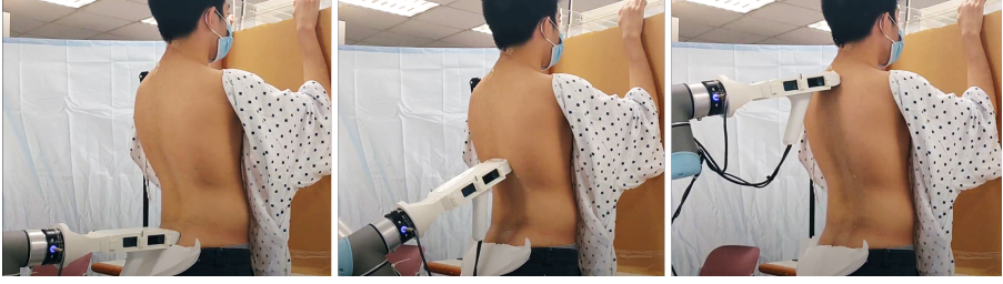
Fig. 4 The images from the robotic scanning procedure video for one of the subjects. The robot adjusts the ultrasound probe rotation according to the force sensing and smoothly scans through the patient's back, maintaining constant contact.
