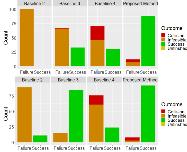
Fig. 4. Comparison of the proposed methods with 3 baseline methods in two intersection scenarios. Here \epsilon \mathcal{N}(0, 0.15) . The confidence level is \eta = 0.9999 . Weights in the objective function for the optimization problem are adjusted for each scenario. In case 2 the nlmpc avoids being between the other two vehicles.
