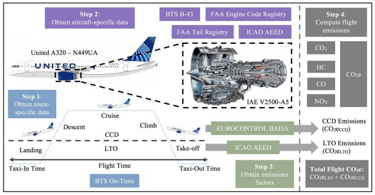
Fig. 3. Graphic workflow of the emissions estimation methodology utilized in the optimization. Each one of the colors (blue, violet, green, grey) represents a different step in the methodology. A total of six different open-source datasets are employed and integrated, including: BTS On-Time, BTS B-43, FAA Engine Code Registry, FAA Tail Registry, ICAO Aircraft Engine Emissions Dataset (AEED) and EUROCONTROL Base of Aircraft Data (BADA).
