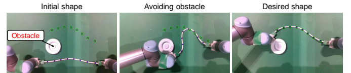
Fig. 23. Case of using the MPC with our Jacobian model for obstacle avoidance. Note that such an approach requires an accurate offline model.
