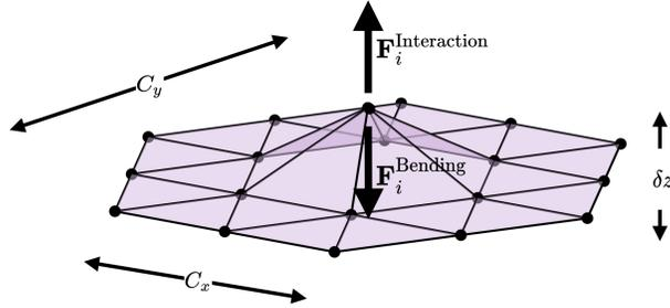
Figure SI.1: Test element used to calibrate model.  $C_x$  and  $C_y$  are the amount of compression in the  $x$  and  $y$  components respectively, and  $\delta z$  the  $z$  displacement from equilibrium.
