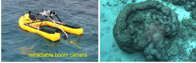
Fig. 5: FloatyBoat is configured with a retractable boom camera (left) for 3D reconstruction of coral reefs. 3D reconstructions of a large coral from Loomis reef (right) generated using imagery collected by the ASV.
