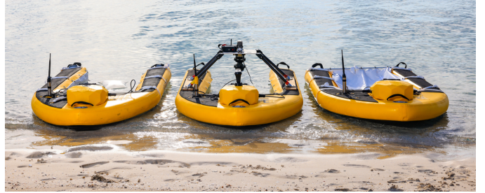
Fig. 1: A sample fleet of modular FloatyBoats configured for capturing coral spawn (left), monitoring and 3D mapping reefs (middle), and deploying coral larvae (right).
