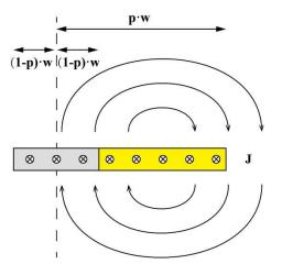
**Fig. S5 Schematic illustration of Oersted field generated by evenly distributed current in Hall bar.** The dashed line marks the calculation position. The grey region marks the region whose net contribution to the Oersted field is canceled out.
