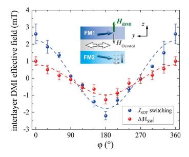
Figure 5. Effective field of interlayer DMI, derived from AHE and SOT switching measurement, respectively. The blue points show the Oersted field at the average boarder between the switching and non-switching regions under 90 MA/cm<sup>2</sup> current pulse. The red points show  $\Delta |H_{SW}|$  of FM1 summarized from AHE experiment. The dotted lines are the fittings using a sine function.
