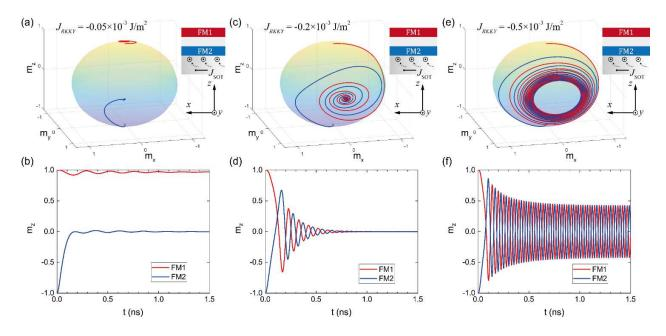
**Fig. S2 Macro-spin simulation of SOT induced magnetization dynamics with different RKKY coupling energy.** 200 MA/cm<sup>2</sup> SOT current is applied and the spin injection is in only the bottom layer. **a-b** SAF precession with  $J_{RKKY}$  = -0.05×10<sup>-3</sup> J/m<sup>2</sup>. **c-d** SAF precession with  $J_{RKKY}$  = -0.2×10<sup>-3</sup> J/m<sup>2</sup>.
