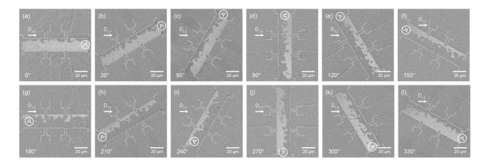
**Fig. S4 Representative Kerr images of SOT switching in different azimuthal directions.** Switching area in Hall bar sample with an azimuthal rotation of 0°(**a**), 30°(**b**), 60°(**c**), 90°(**d**), 120°(**e**), 150°(**f**), 180°(**g**), 210°(**h**), 240°(**i**), 270°(**j**), 300°(**k**), 330°(**l**). The injection direction of current pulse is marked at one port of the current channel.
