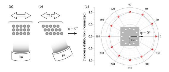
**Fig. S1 Thickness distribution during the slanted epitaxial film growth. a-b** Schematic illustration of face to face (a) and slanted (b) magneton sputtering. **c** Thickness distribution among the sample, normalized by the thickness of the center point. Inset shows the distribution of test points.
