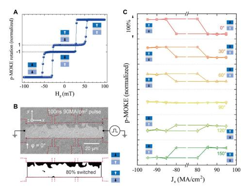
Figure 4. Field-free SOT switching detected by optical Kerr measurement. (A) Normalized p-MOKE signal of the studied film. (B) Kerr image after the application of a current pulse. The switching area is counted from the composite image below. (C) Summarization of current induced switching behavior as a function of  $\varphi$ . As shown in (B), the direction of  $\varphi$  is along the voltage channel of the Hall bar device.
