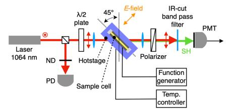
Supplementary Fig. 27 | The optical setup for SHG studies. The electric field (*E*-field) was applied normal to the sample cell (thickness: 5  $\mu$ m), generating the *p*-in/*p*-out polarization combination.
