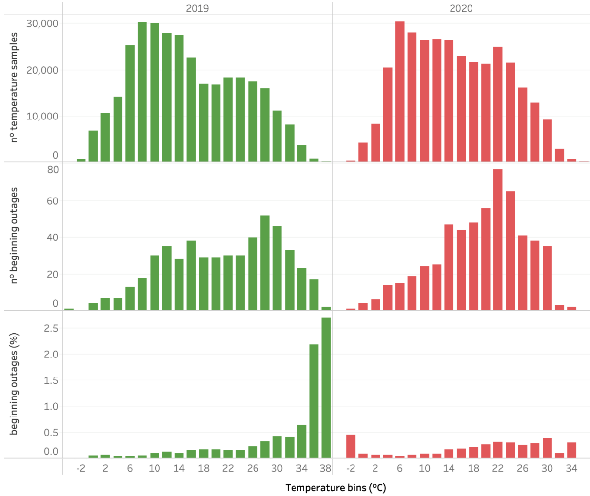
Fig. 16. Upper graph: number of temperature samples per temperature bin. Middle graph: number of outages begun within the temperature bin. Lower graph: percentages of outages begun within the temperature bin over the total number of temperature samples in the bin.
