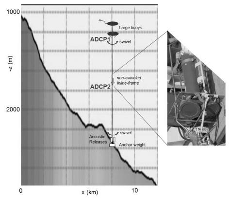
**Figure 1.** Mooring outline sketch over partial Mount Josephine bathymetry from east-west Multibeam transect along 37 °00′N. The bathymetry aspect ratio vertical:horizontal is 8:1. The photo shows the inline-frame with the deep-water ADCP.
