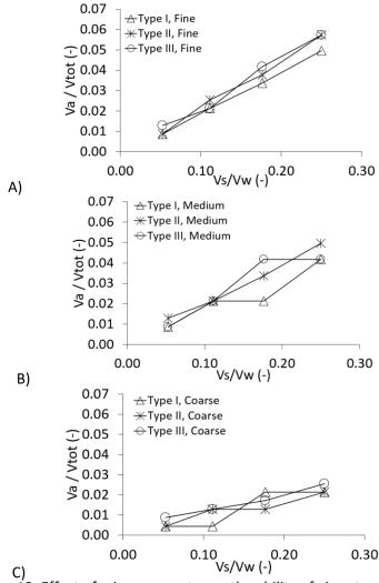
Figure 13. Effect of mixer geometry on the ability of air entrapment.
