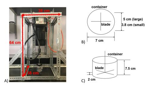
Figure 14. Illustrations for: A) mixing station; B) plan view and dimension of the mixing container; C) front view and dimension of mixing container
