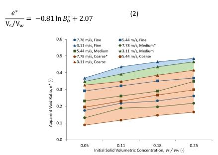
Figure 6. Coupled effect mixing speed and types of sand particles on the ability to trap air phase for different sand particle sizes. The Star sign indicates the average results for multiple tests under the same conditions.
