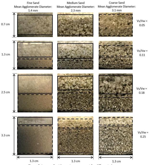
Figure 9. Layers of settlement arrangement for different phases.
