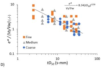
Figure 5. Coupled effect mixing time and types of sand particles on the ability to trap air phase for A) fine sand particles, B) medium sand particles, D) coarse sand particles, and D) combined results.
