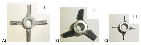
Figure 12 Mixing blade geometries considered for the experiments: A) Type I with 5 cm span, B) Type II with 4 cm span.
