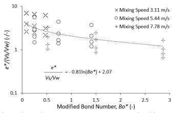
Figure 7. Empirical correlation between air entrapment normalized by initial solid volumetric concentration and modified Bond Number.
