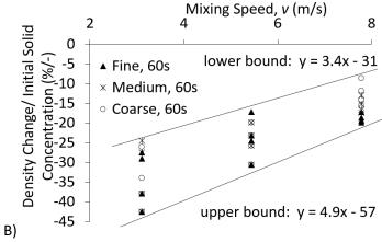
Figure 8. Density reduction because of A) mixing time and B) mixing speed.
