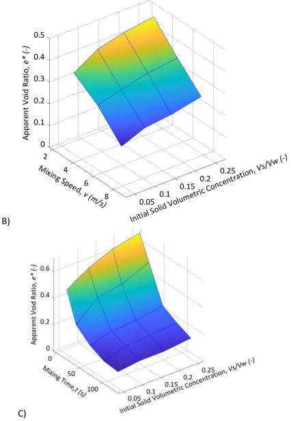
Figure 4. Coupled effect of initial solid volumetric concentration and other factors including A) type of sand particles, B) mixing speed, and C) mixing time on the ability to trap the amount of air phase. Results are shown in the intersection of mesh lines.
