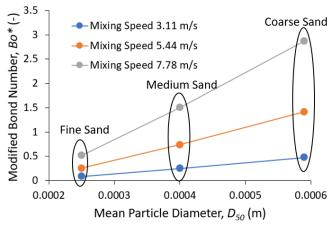
Figure 3. The combined effect of mean particle diameter and mixing speed on the modified Bond Number.
