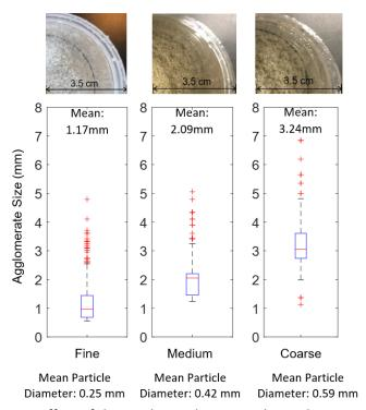
Figure 2. Effect of the sand particle size on the agglomerate size.
