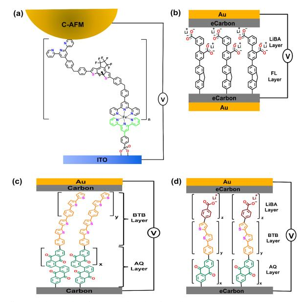
**FIG. 3 Schematic illustration of molecular junctions featuring** (a) (Fe-tpy-DTE-tpy)<sub>n</sub> multilayer assembled via LbL technique; (b) FL<sub>4.5</sub>/LiBA<sub>4</sub> bilayer; (c) BTB/AQ bilayer; and (d) a LiBA/BTB/AQ trilayer. The molecules were assembled on either ITO (a) or eCarbon/Au (b-d) substrates; a CP-AFM tip (a) or eCarbon/Au (b-c) were used as the top electrode.
