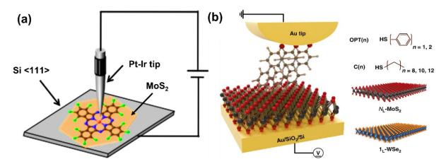
FIG. 4 Schematic illustration of molecular junctions featuring (a)  $MoS_2/MPc$  (metal-phthalocyanines), and (b)  $MoS_2$  or  $WSe_2$  /SAMs heterostructures for studying nanoscale rectification. Figures (a) and (b) are reproduced with permission from ref.<sup>143</sup> and ref.<sup>144</sup>, respectively.
