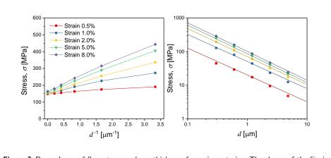
Figure 3 Dependency of flow stress on layer thickness for various strains. The slopes of the fits in the double-logarithmic plot on the right graph indicate a Hall-Petch exponent between  $\delta = 0.8$  and  $\delta = 0.85$ .
