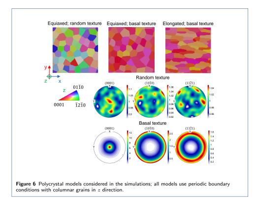
grain size d is then defined via  $L^2 = Nd^2$  where L is the physical size of the model. The grain size is varied by scaling L, hence, the spatial resolution at which the grain microstructure is captured is always the same.
