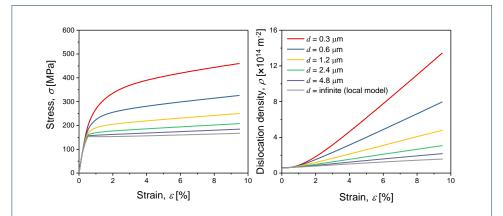
**Figure 2** Left: Stress-strain curves of bicrystal multilayers for five different layer thicknesses; right: evolution of average dislocation density for the same samples. For reference, we also show results for a model without transport or back stress, corresponding to layer thicknesses that are so large that boundary effects near the layer boundary can be neglected.
