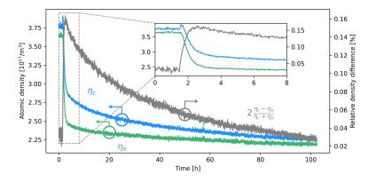
**Figure 5.** Retrieved atomic densities at the center (blue) and edges (green) of a 60 µm Kagomé fibre when decreasing the reservoir temperature from 65 to 45 °C while keeping a constant cell temperature of 80 °C. The grey curve is the relative density change  $2(\eta_c - \eta_e)/(\eta_c + \eta_e)$ .
