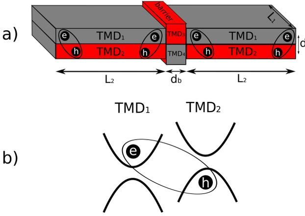
FIG. 1. (a) Schematic of Josephson junction with the different layers labelled TMD<sub>1</sub>–TMD<sub>4</sub>.  $d$  is layer separation,  $d_b$  the barrier thickness, and  $L_1$  and  $L_2$  the transverse and longitudinal layer lengths. Electron-hole pairs are shown. (b) Energy band alignments at the type-II TMD<sub>1</sub>/TMD<sub>2</sub> interface.
