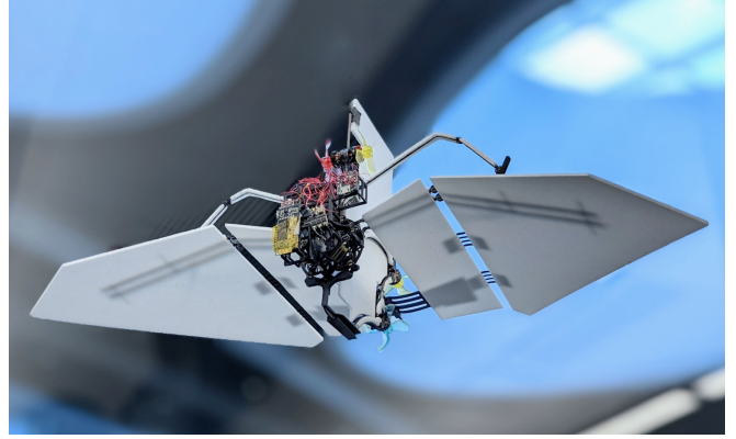
Fig. 1. Shows Northeastern University’s morphing wing robot, Aerobat . Aerobat is employed to test our bang-bang flight control.
