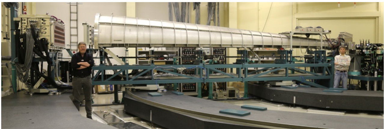
Figure 2: The high-resolution spectrometer at BL43LXU. Samples are placed on the stages at the far right and the meV analyzers are in the chamber at the far left. Two scientists (A. Baron, left, and D. Ishikawa, right) are shown for scale.
