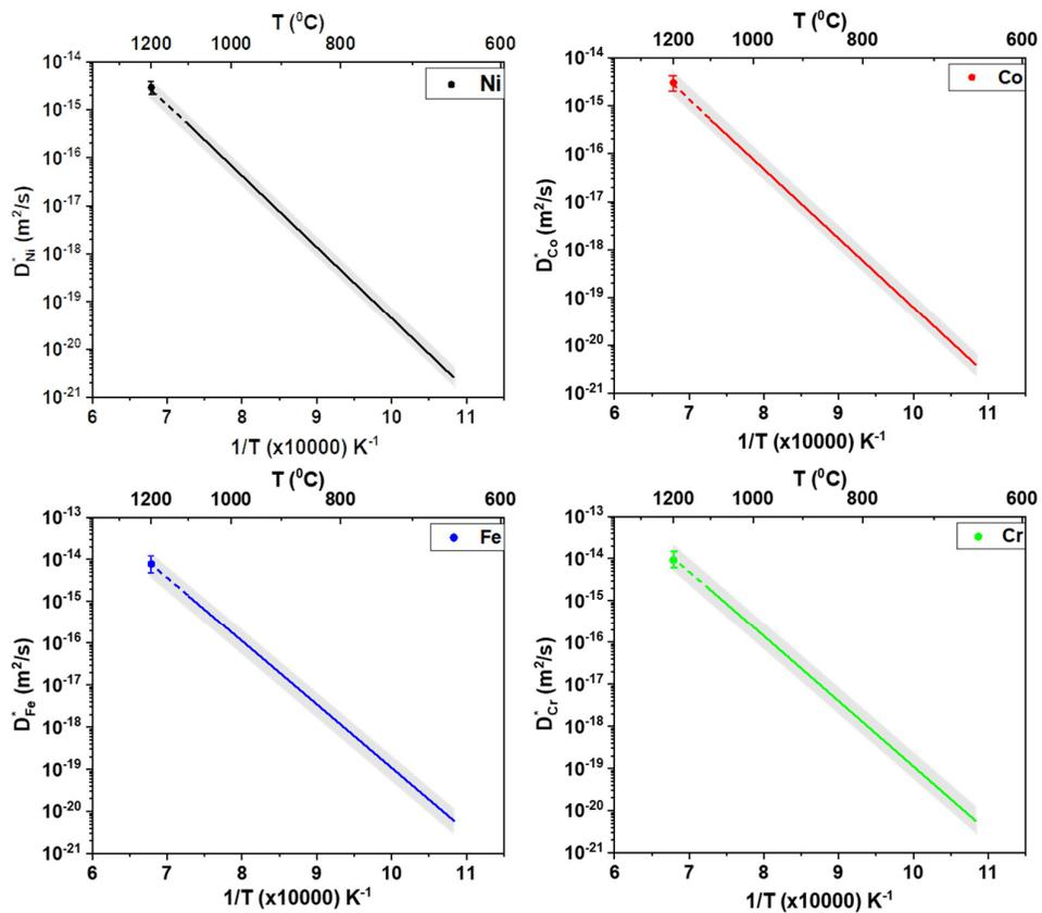
Fig. 3: Comparison of tracer diffusion coefficients estimated following the radio-tracer method [21] with the data estimated following the pseudo-binary, pseudo-ternary and body-diagonal diffusion couple methods.
