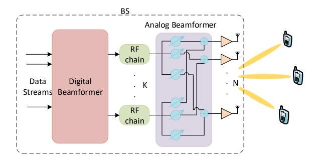
Fig. 1: mmW-NOMA system diagram for joint power allocation and hybrid beamforming
