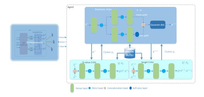
Fig. 2: Schematic diagram of soft actor-critic network
