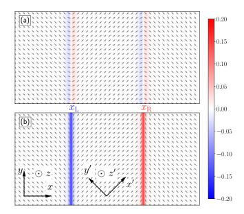
FIG. 1. 90° magnetic DWs resulting from micromagnetic simulations: (a) uncharged DWs, (b) charged DWs. The color scale shows the z-component of reduced magnetization vector  $\boldsymbol{m} = \boldsymbol{M}/M_{\rm s}$ . The parameters of calculation were  $A_{\rm ex} = 1.3 \times 10^{-11} \, {\rm J/m}, M_{\rm s} = 7.20 \times 10^5 \, {\rm A/m}, K_u = 10^4 \, {\rm J/m}^3$ , and  $D = 2 \, {\rm mJ/m}^2$ . The distance between the domain walls is  $x_{\rm R} - x_{\rm L} = 1 \, \mu m$ .
