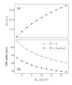
FIG. 3. Dependence of (a) the out-of-plane magnetization,  $m_z(x_c)$ , and (b) the DW width of a charged 90° DW as a function of the anisotropy constant,  $K_u$ . The parameters used in the calculations are the same as in Fig. 1. Calculations of  $m_z(x_c)$  were done with  $D = 2 \text{ mJ/m}^2$ ;  $x_c$  is the position of the anisotropy boundary. DW width has been calculated with and without DMI.
