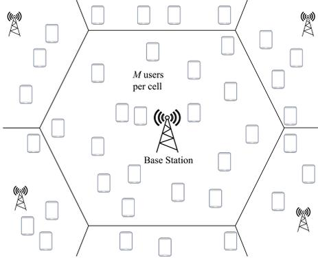
Fig. 1: An uplink MC system with  $Q$  cells.
