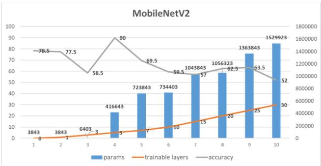
Fig 10. MobileNetV2 Accuracy vs Trainable Layers vs Parameters
