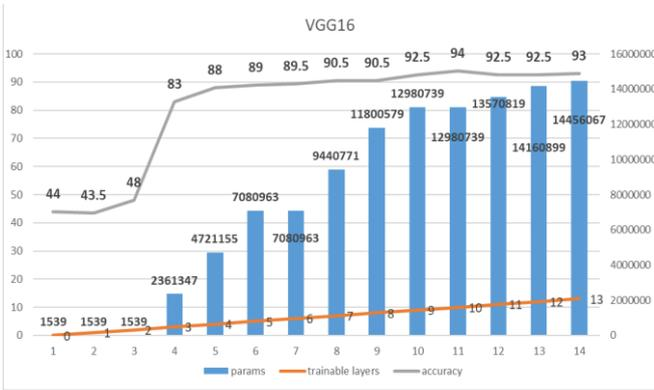
Fig 9. VGG16 Accuracy vs Trainable Layers vs Parameters
