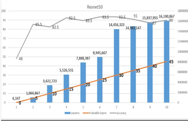
Fig 8. Resnet50 Accuracy vs. Trainable Layers vs. Parameters
