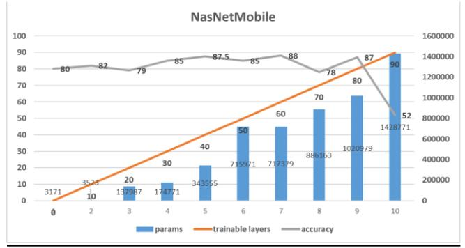
Fig 11. NasNetMobile Accuracy vs. Trainable Layers vs. Parameters
