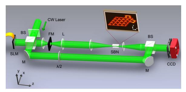
Fig. S4. Schematic illustration of the experimental setup employed for writing and probing a photonic lattice in a photorefractive crystal. SLM: spatial light modulator; BS: beam splitter; FM: Fourier mask; L: circular lens; SBN: strontium barium niobite crystal; M: mirror;  $\lambda/2$ : half-wavelength plate; CCD: charge-coupled device.
