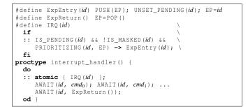
Figure 3: An Interrupt Handler Model
