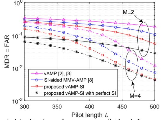
Fig. 2. Activity detection performance versus pilot length  $L$ .
