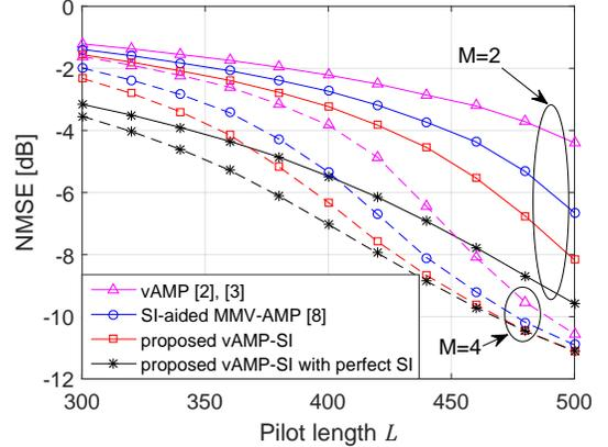
Fig. 3. Channel estimation performance versus pilot length  $L$ .
