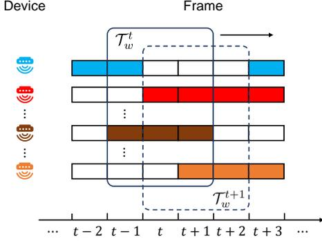
Fig. 1. The diagram of the sliding-window detection strategy
