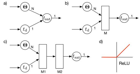
FIG. 1. a)-c) Shallow and deep neural networks considered in this work d) rectifying linear function (ReLU) used in each of the layers.
