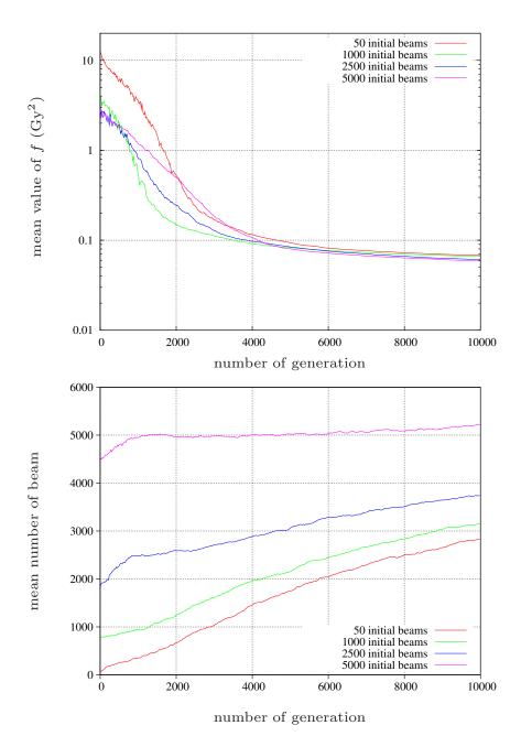
Figure 4: Influence of the initial beam number on the evolution process. The convergence of the objective function (top) and the evolution of the mean number of coding beams (bottom) are represented for 50, 1000, 2500 and 5000 initial beams.
