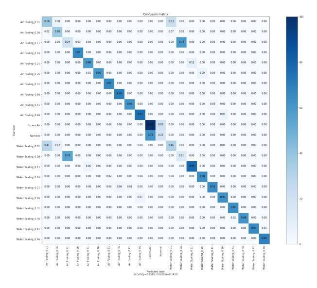
Figure 7. Vitorond 950 – Random Forest with Single Excess Air Class {'bootstrap': True, 'Maximum Depth': None, 'Maximum Features': 5, 'Minimum Leaf Samples': 1, 'Minimum Split Samples': 2, 'Number of Estimators': 100}
