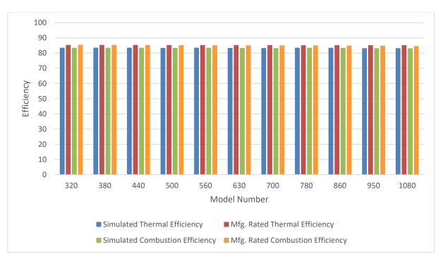
Figure 4. Viessmann Vitorond 200 Thermal and Combustion Efficiency
