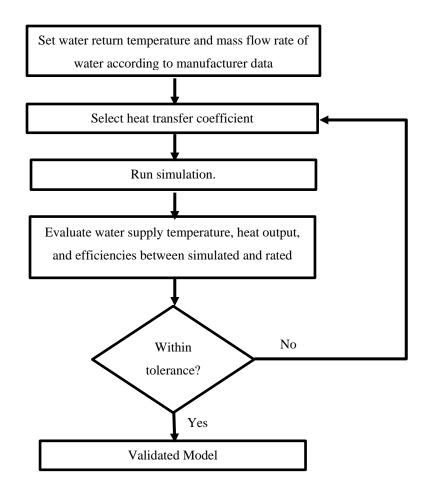
Figure 2. The iterative approach used for calculating gas-side heat transfer coefficient
