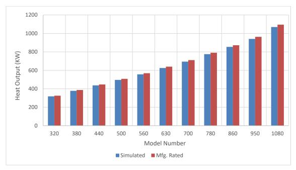
Figure 3. Viessmann Vitorond 200 Boiler Series Thermal Output
