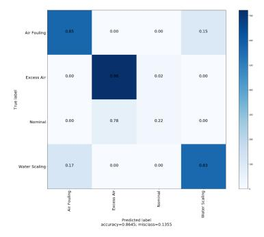
Figure 8. Vitorond 950 – Random Forest with 4-class classification {'bootstrap': True, 'Maximum Depth': None, 'Maximum Features': 5, 'Minimum Leaf Samples': 1, 'Minimum Split Samples': 4, 'Number of Estimators': 500}
