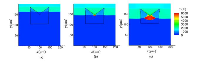
Figure 6. (a) – (c). A sequence of temperature contours obtained from the numerical calculation for  $U_p = 2500$  m/s shock interacting with a representative HMX crystal with  $\theta = 90^{\circ}$  embedded in Estane.
