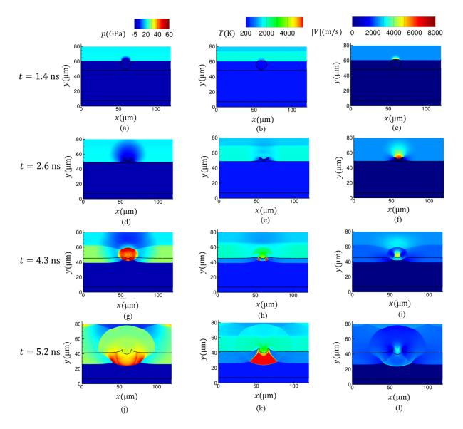
Figure 14. Sequence of contours of pressure (left column), temperature (middle column), and velocity magnitude (right column) at four different instances during the  $U_p = 2500$  m/s shock interaction with a void (14 µm in diameter) in the binder located near the crystal-binder interface.
