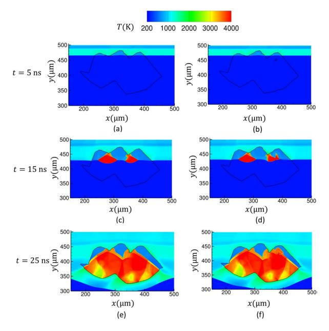
Figure 28. Sequence of temperature contours during a  $U_p = 2300$  m/s shock interaction with an imaged geometry of a HMX crystal embedded in Estane binder.
