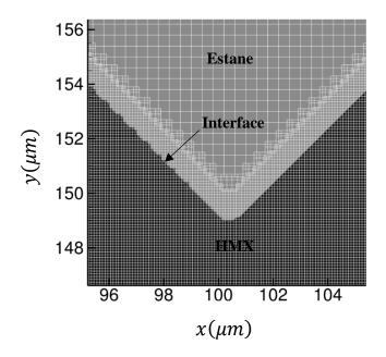
Figure 4. Locally refined mesh around the interface of HMX crystal and Estane binder.
