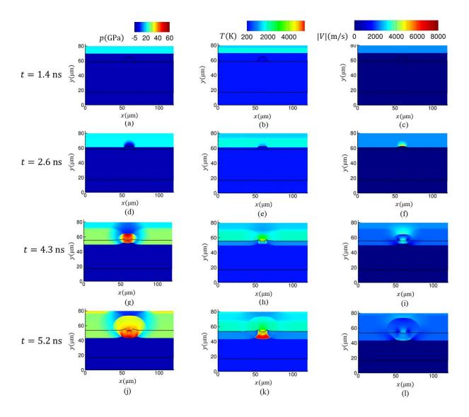
Figure 12. Sequence of pressure (left column), temperature (middle column), and velocity magnitude (right column) contours at four different instances during the  $U_p = 2500$  m/s shock interaction with a semi-circular delamination at the crystal-binder interface.
