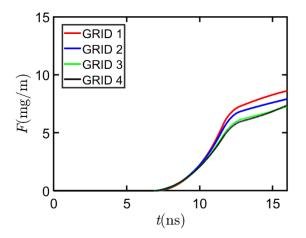
Figure 5. A grid sensitivity study: comparison of F computed using different grid resolutions  $(\Delta x_{\text{base}} = 1.6 \,\mu\text{m}, 0.8 \,\mu\text{m}, 0.4 \,\mu\text{m}, \text{and } 0.2 \,\mu\text{m})$
