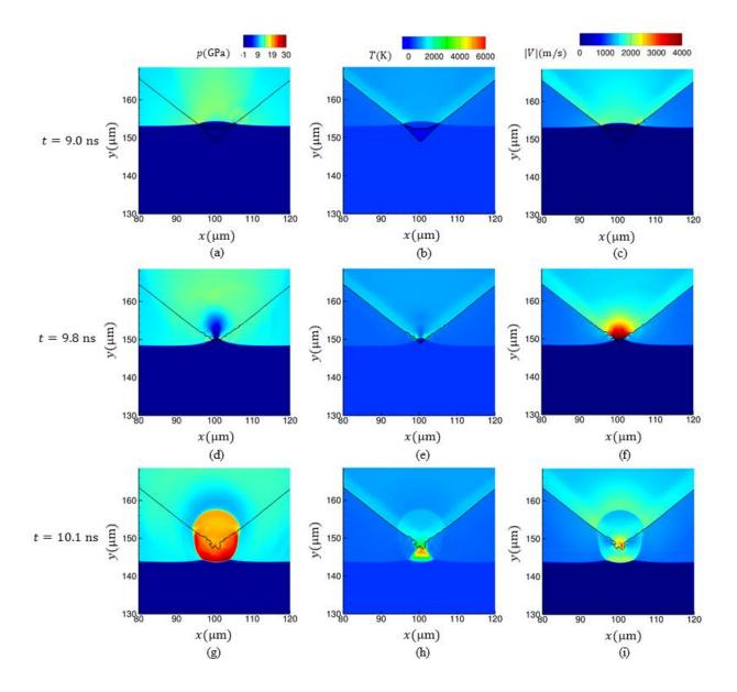
Figure 10. (a) – (i). A sequence of temperature contours obtained from the numerical calculation for  $U_p = 1500 \text{ m/s}$  shock,  $\theta = 90^0$  and with a delaminated region of 9 µm radius of curvature at the corner. The rows from top to bottom correspond to the times 9.0 ns, 9.8 ns, and 10.1 ns respectively. The columns from left to right show the contours of pressure, temperature, and velocity magnitude, respectively.
