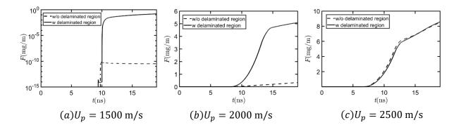
Figure 11. Comparison of *F* vs *t* with and without a delaminated region (see Figures 3 (a) and (b) respectively). The response of the crystals with and without the delaminated region at the corner to  $U_p = 1500 \text{ m/s}$ , 2000 m/s, and 2500 m/s shocks are compared in (a), (b), and (c) respectively.
