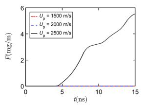
Figure 13. Comparison of F vs t during  $U_p = 1500$ , 2000, and 2500 m/s shock interaction with a semi-circular delamination region at the crystal-binder interface.
