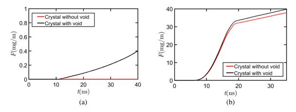
Figure 17. The comparison of F vs t during interaction of the shock with HMX crystal, for a crystal with and without a void at (a)  $U_p = 1500$  m/s and (b)  $U_p = 2300$  m/s.
