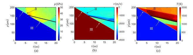
Figure 7. y - t plots of (a)pressure, (b) velocity component along the y-axis and (c) temperature obtained from non-reactive calculation of the  $U_p = 2500$  m/s shock interaction with the HMX crystal with  $\theta = 90^{\circ}$  embedded in binder. The trajectory of the interface is marked with the black line. The markers (I), (II), and (III) show the incident, transmitted, and reflected waves, respectively.
