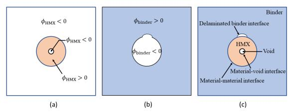
Figure 2. A schematic diagram of a circular HMX crystal with a void at its center embedded in binder to demonstrate the sign convention used to define separate levelset fields describing the crystal and the binder region. (a) shows the levelset field for HMX crystal, (b) shows the levelset field for binder, and (c) shows the crystal-binder interface with a delaminated region.
