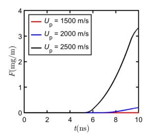
Figure 15. Comparison of F vs t for  $U_p = 1500$ , 2000, and 2500 m/s, shock interaction with a void (14 µm in diameter, centered at 15.4 µm away from the interface) in the binder located near the crystal-binder interface.
