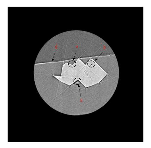
Figure 1. CT scan of HMX crystal in binder. Noticeable features of the HMX crystal: (a) sharp corner at crystal-binder interface, (b) void in HMX crystal, (c) debonding between the crystal and binder at the interface, and (d) binder air interface.
