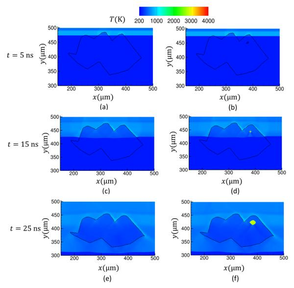
Figure 16. Sequence of temperature contours during a  $U_p = 1500$  m/s shock interaction with an imaged geometry of HMX crystal embedded in Estane binder.
