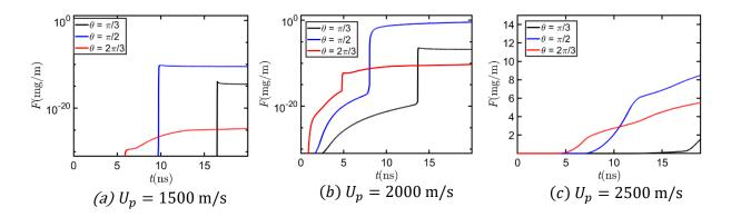
Figure 9. Comparison of the amount of final combustion product(*F*) produced in the 2D plane of calculation during shock interaction with synthetic HMX crystals with  $\theta = 60^{\circ}$ ,  $90^{\circ}$ , and  $120^{\circ}$  shown in Figures 3. The response of the three crystals to  $U_p = 1500 \text{ m/s}$ , 2000 m/s, and 2500 m/s shocks are compared in (a), (b), and (c) respectively.
