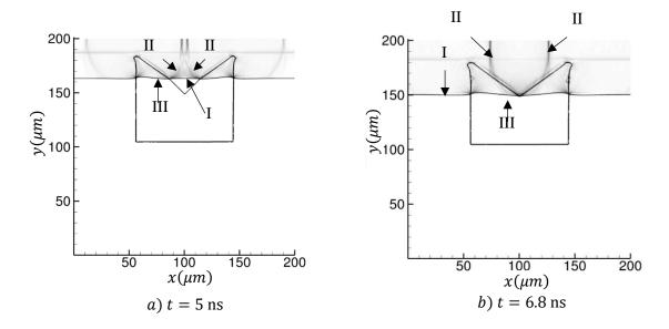
Figure 8. Numerical Schlieren at a) 5 ns and b) 6.8 ns during the  $U_p = 2500$  m/s shock interaction with the representative HMX crystal (chemically inert) with  $\theta = 90^0$  embedded in Estane binder. The numerical Schlierens show reflected waves (II) generated due to the interaction of the interaction of the incoming shock (I) with the wedge shaped crystal-binder interfaces. The wave transmitted within the crystal is marked with (III).
