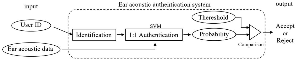
Figure 2: Overview of ear acoustic authentication system
