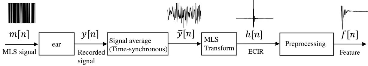
Figure 6: The flow of data measurement and preprocessing
