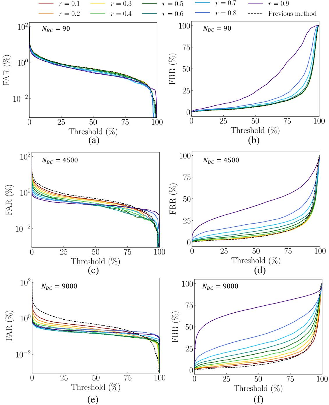
Figure 9: FAR and FRR curves with various parameters. (a) FAR curve of  $N_{BC} = 90$ . (b) FRR curve of  $N_{BC} = 90$ . (c) FAR curve of  $N_{BC} = 4500$ . (d) FRR curve of  $N_{BC} = 4500$ . (e) FAR curve of  $N_{BC} = 9000$ . (f) FRR curve of  $N_{BC} = 9000$ .
