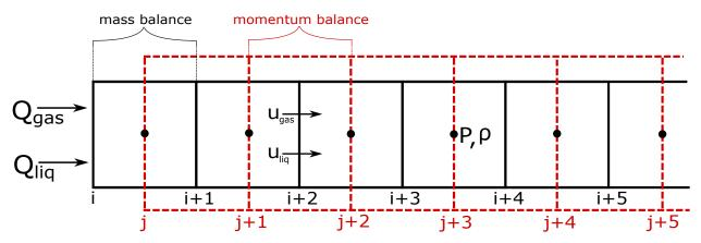
Figure 4: Staggered grid discretization scheme used to solve the system of equations of the drift-flux model
