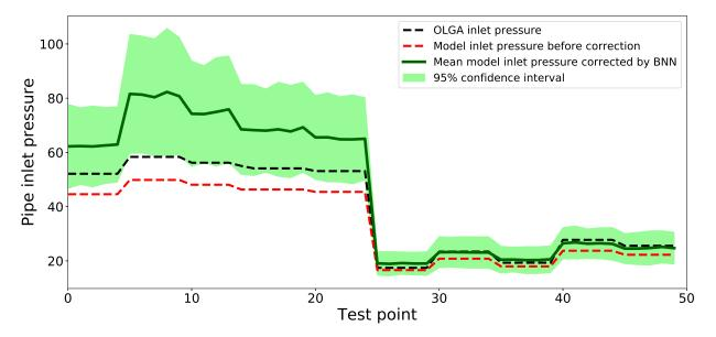
Figure 10: Estimated mean and 95% confidence interval of the corrected multiphase flow model using Bayes by Backprop Bayesian Neural Network Case 2.
