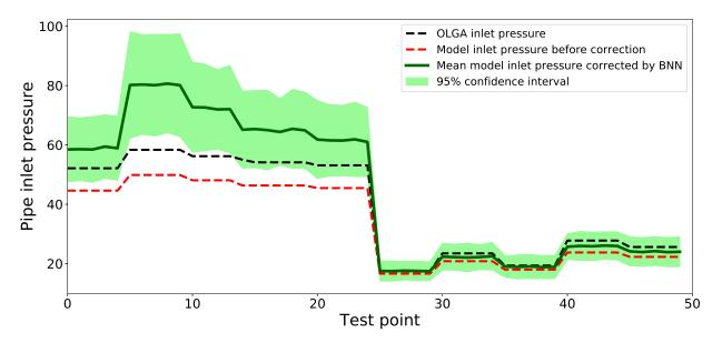
Figure 9: Estimated mean and 95% confidence interval of the corrected multiphase flow model using MC Dropout Bayesian Neural Network for Case 2.
