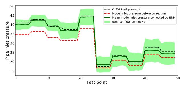
Figure 7: Estimated mean and 95% confidence interval of the corrected multiphase flow model using MC Dropout Bayesian Neural Network for Case 1.
