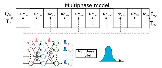
Figure 6: Prediction stage of Bayesian Neural Networks for predicting the mean and variance of the modeled variable
