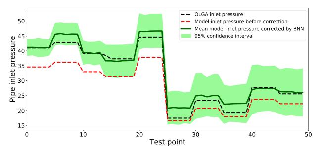
Figure 8: Estimated mean and 95% confidence interval of the corrected multiphase flow model using Bayes by Backprop Bayesian Neural Network Case 1.
