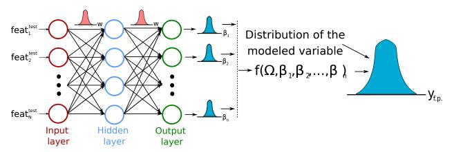
Figure 2: Prediction stage of Bayesian Neural Networks for predicting the mean and variance of the modeled variable
