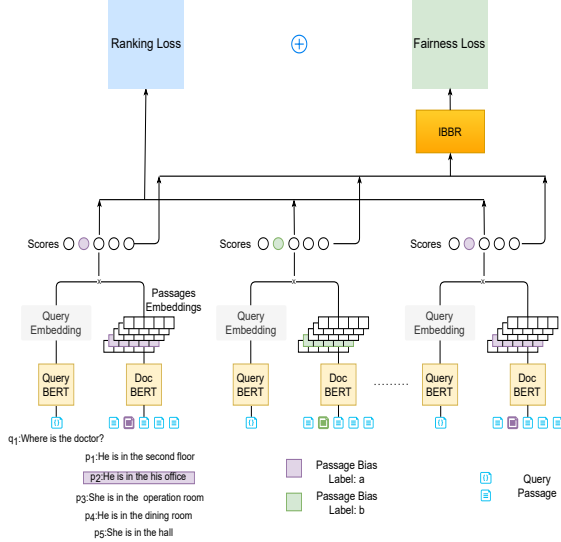
Figure 1: An example of In-Batch Balancing Regularization method. For each query, we calculate the typical ranking loss and the fairness loss from IBBR on top K retrieved passages. We jointly optimize the ranking loss and the fairness loss. There are two ways of computing the IBBR, pairwise difference loss and T-statistics Loss.
