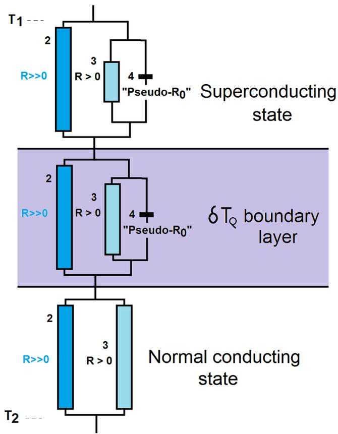
**Figure 7** Resistances of a stack of thin films (schematic) with solid/solid contacts. The Figure, from top to bottom, simulates a standard, superconductor/normal conductor/superconductor sequence. For the simulation of Andreev reflection, layer 2 (mid-position) is normal conducting. Transition from superconducting to normal conducting resistivity is indicated by a  $\delta T_Q$  resistive boundary layer, a temperature uncertainty extending over given geometrical layer thickness. Compare text.
