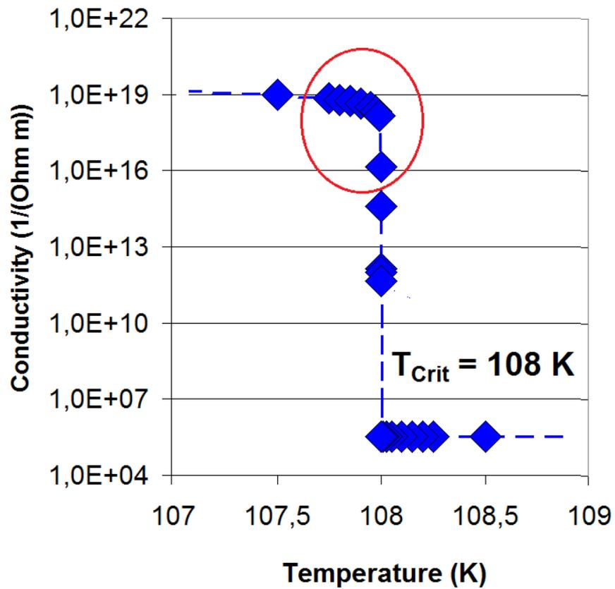
Figure 6c Electrical conductivity,  $1/\rho_{\text{El,SC}}$ , of BSCCO 2223 calculated from the resistivity values shown in Figure 6a. The red circle highlights bending of the curve that here is more clearly seen than in Figure 6a,b.
