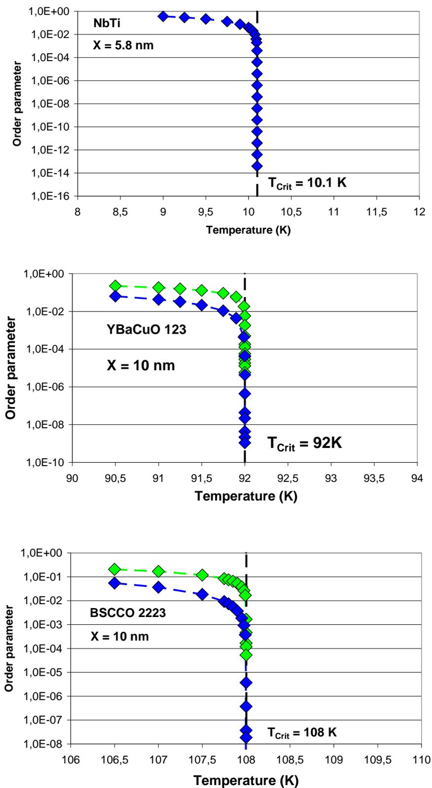
**Figure 3** Order parameter,  $f_S = n_S(T)/n_S(T=4K)$  of NbTi, YBaCuO 123 and BSCCO 2223 vs. temperature. Results are obtained using either the microstability model [7] or the approximation Eq. (8) of [9] (light-green and blue symbols, respectively).
