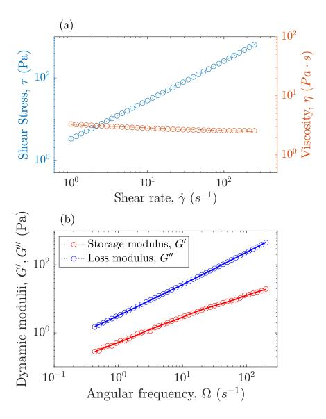
FIG. 2: Rheology of the BF-II fluid: (a) shear stress vs shear rate for the viscosity measurement; (b) oscillation test for the relaxation time measurement, storage modulus (red circls) and loss modulus (blue circles) vs oscillating frequency  $\Omega$ . The solid lines show the fit to the data using the generalised Maxwell model Eq. 2.
