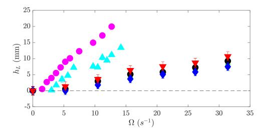
FIG. 3: Levitation height,  $h_{\rm L}$  (mm), as a function of the rotational speed,  $\Omega$  (s<sup>-1</sup>) for the Boger fluids (BF-I and BF-II). The symbols for each experiment correspond to those in Table I. The dashed line shows the measurements for the Newtonian case (no levitation observed).
