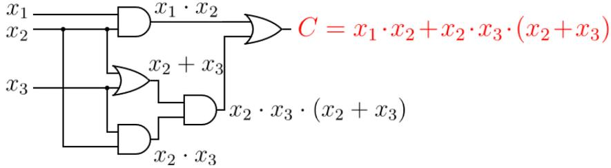
Figure 1: An arithmetic circuit  $C$  that realizes the function  $f(x_1, x_2, x_3) = x_1 \cdot x_2 + x_2 \cdot x_3 \cdot (x_2 + x_3)$ .
