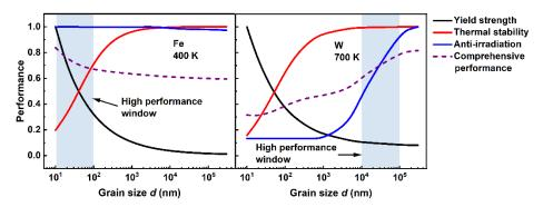
**Fig. 7. Comprehensive performance prediction for Fe- and W-based materials.** High-performance windows for Fe and W, when considering the synergy of thermal stability, mechanical property (yield strength), anti-irradiation ability with different grain sizes. Here, the
