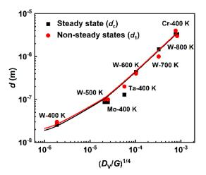
**Fig. 6. Critical grain sizes.** The comparison of the relationship of  $d_c$  and  $d_1$  with  $(D_v/G)^{1/4}$  in both the steady state and non-steady states.
