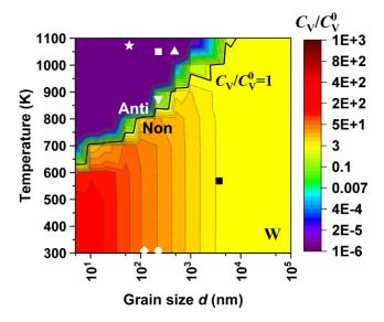
Fig. 4. Radiation resistant window after annealing. Verification of radiation resistant window of CD predictions with experiments (19-21, 25, 46, 47) for W under uniform
