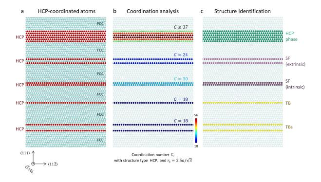
Fig. S4. Deformation SF, hcp phase, and twin boundary identification. a, A fcc structure containing hcp-coordinated atoms. b, Atoms are colored by weighted coordination number Z, that measures the number of same hcp-structure neighbors an atom has within a cutoff distance  $2.5a/\sqrt{3}$  (here a is the lattice constant). c, All the hcp structures, including intrinsic SF (iSF), extrinsic SF (eSF), TB, and hcp phase are identified from Z ( $Z_{TB} = 18$ ,  $Z_{eSF} = 18$ ).
