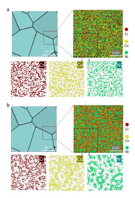
**Fig. S1.**Structures and element distributions in RSS (a) and SRO (b) CrCoNi alloys. The bottom panel in each figure, corresponding to the magnification of the local region (black dotted box), shows the concentration distribution of individual elements, Cr, Co, and Ni.
