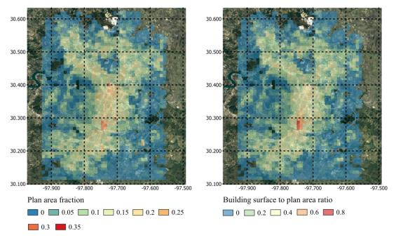
Figure 5. Plan area fraction and building surface to plan area ratio derived from GLOBUS at 1-km resolution over Austin.
