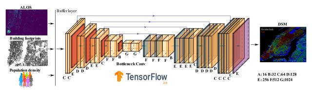
Figure 2. Schematic of UNET-based GLOBUS deep network for generation of building heights.
