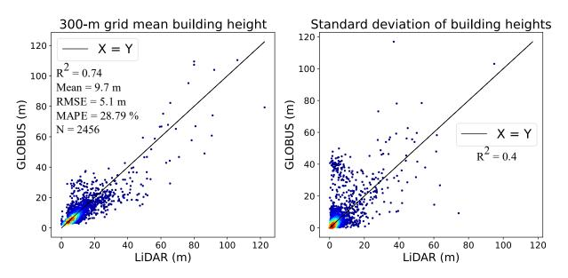
Figure 3. Scatter plots showing the validation of GLOBUS using LiDAR as the ground truth at 300-m spatial resolution.
