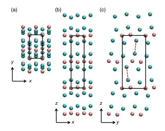
**Fig. S1.** Atomic structure of bulk Td-WTe<sub>2</sub>. The orange and green spheres denote W and Te atoms, respectively, projected toward the (a) z, (b) y, and (c) x directions. The black rectangles indicate the unit cells. The red broken lines are the guidelines representing the alignment of layer stacking.
