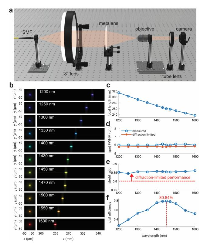
Figure 4. Focusing performance of the fabricated metalens. (a) A schematic of the experimental setup for characterizing the focusing performance of the metalens. The laser out-
