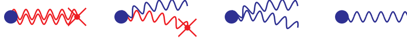
FIG. 5: The diagrammatic representation for the terms of the gluon field strength tensor in the glueball current. The double red line is used for the vacuum gluon field strength tensor G_{\mu\nu}^a . The single red line with the cross at the end denotes the vacuum gluon field. The single blue line denotes the quantum gluon field. The blue lines are part of the coefficient function and the red lines form a condensate.
