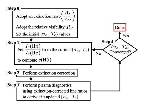
**Figure 1.** A flow chart of PPAP [11], through which converged  $n_e$  and  $T_e$  are sought by a streamlined numerical iterative process given the selection of the extinction law and the corresponding  $R_V$  value as well as the diagnostic line pairs.
