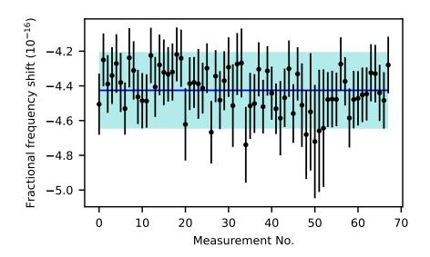
**Figure S2: Micromotion-induced frequency shift.** The shown fractional second order Doppler shift derived from micromotion data was taken during the frequency measurement using <sup>40</sup>Ar<sup>13+</sup>, which had a total measurement duration of around 100,000 s split over several days. The blue line indicates the mean value and the shaded area shows the estimated 68% confidence interval based on the single measurement uncertainty and the standard deviation of the data.
